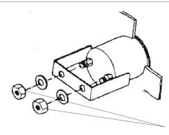
Do not over tighten bolts when installing U bracket. Doing so will cause damage to movement inside.
