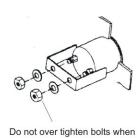
installing U bracket. Doing so will cause damage to movement inside.
