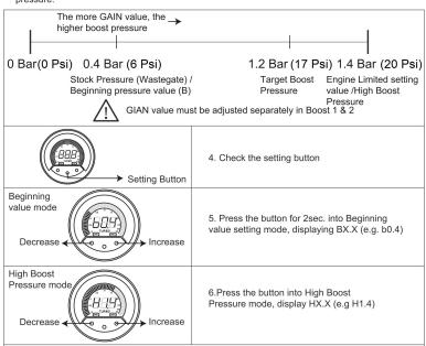
Enter into setting mode, press the ahead right button to decrease 0.1 bar, press left one to increase 0.1 bar
