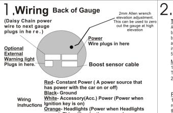
are on). This will make the gauge change color when the headlights are turned on.
